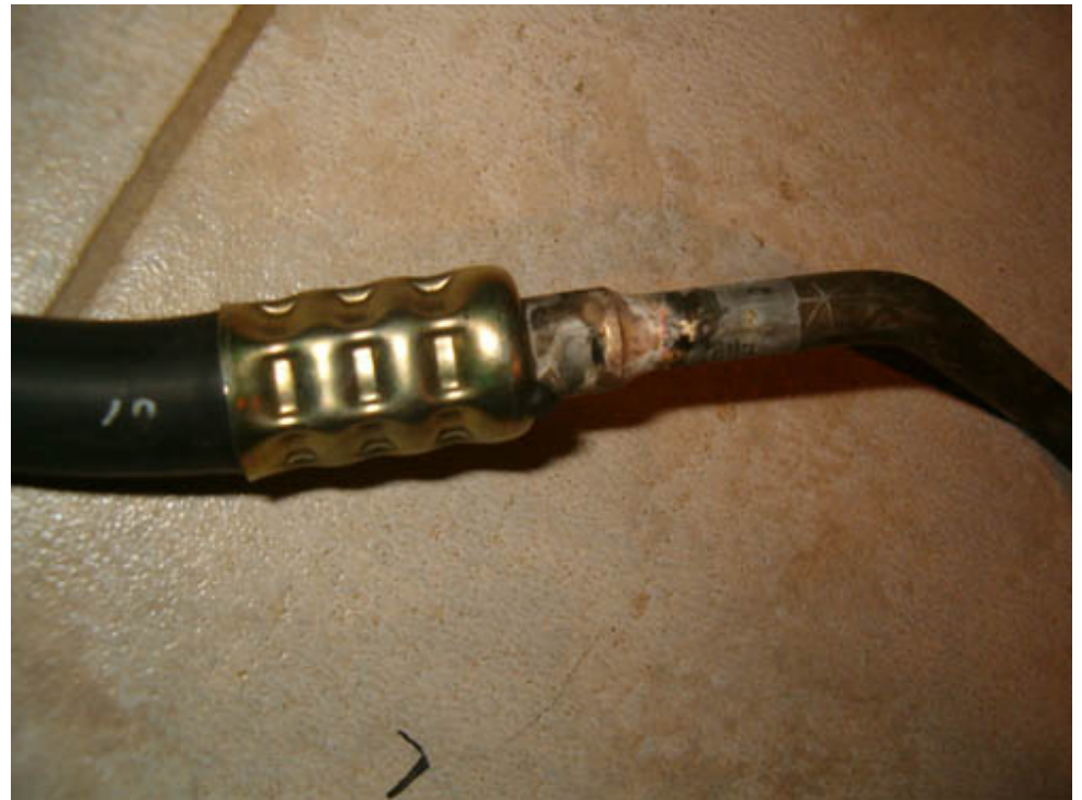
New hose connecting right condenser to drier filter.
