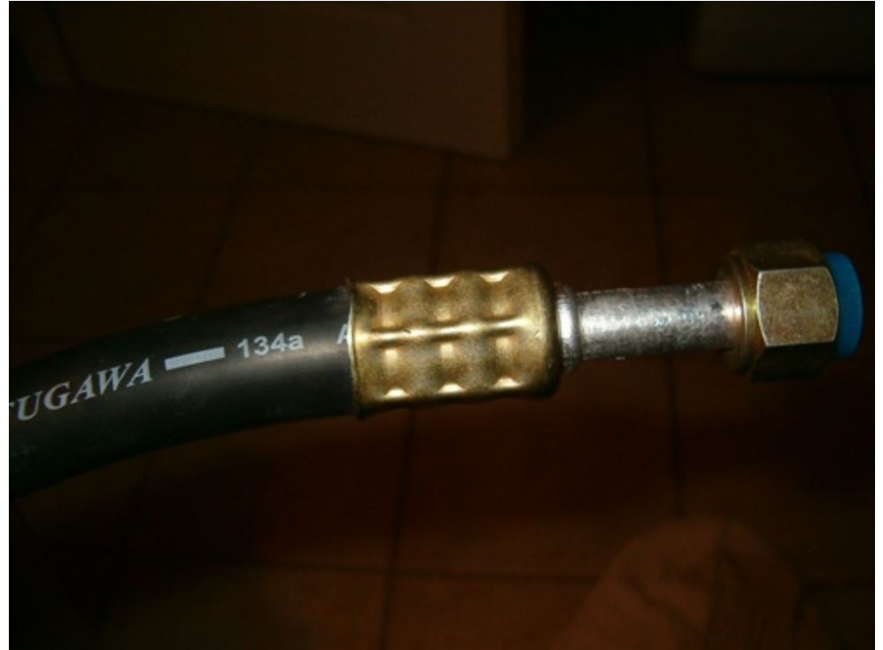
Newly manufactured hose connecting left and right condenser. Notice the designation for use with R134a
