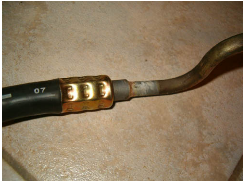
The metal pipe from the original hose was preserved and new R134a hose was used. Notice the welding done in order to adopt new hose and old pipe
