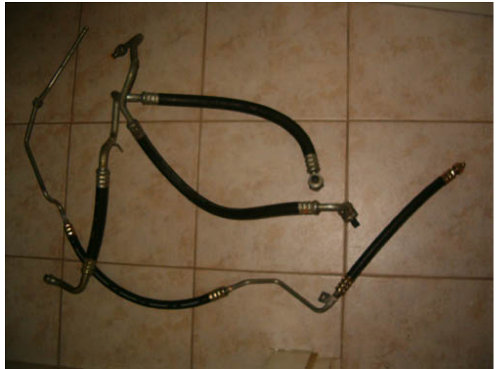
Overview of the hoses. Not showed on the photo is hose running from drier filter to evaporator.
