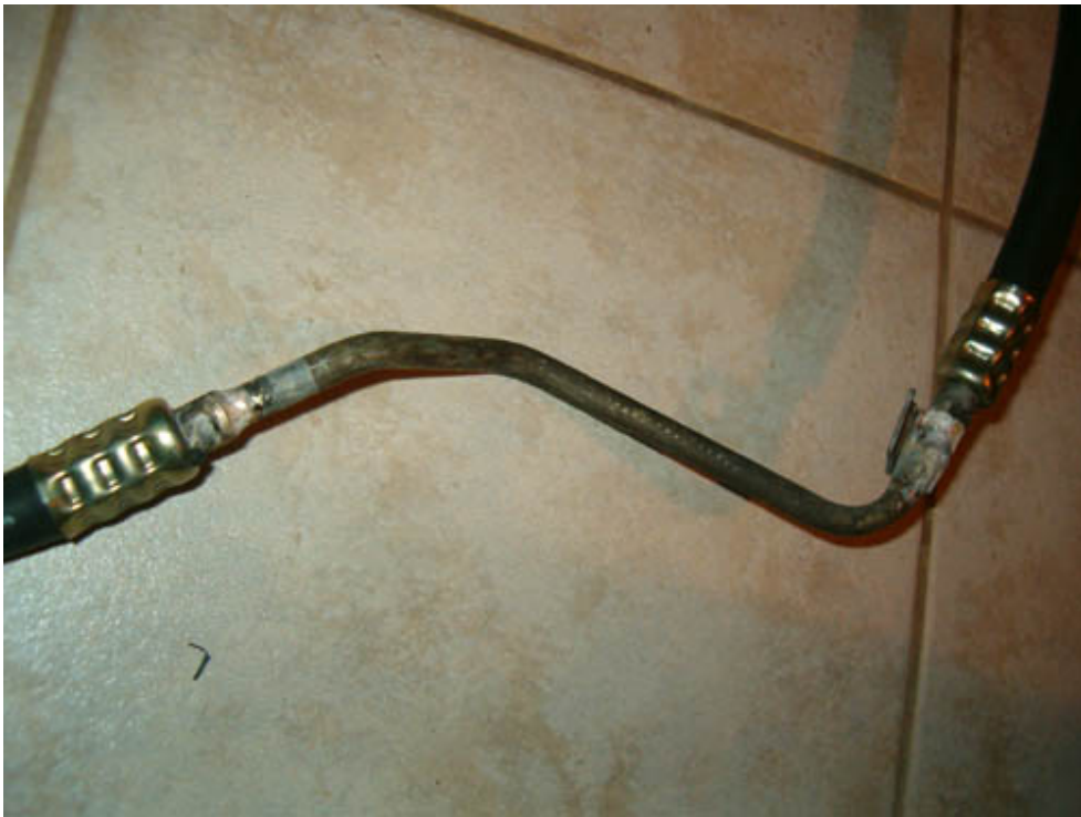
The metal pipe from the original hose was preserved and new R134a hose was used. Notice the welding done in order to adopt new hose and old pipe
