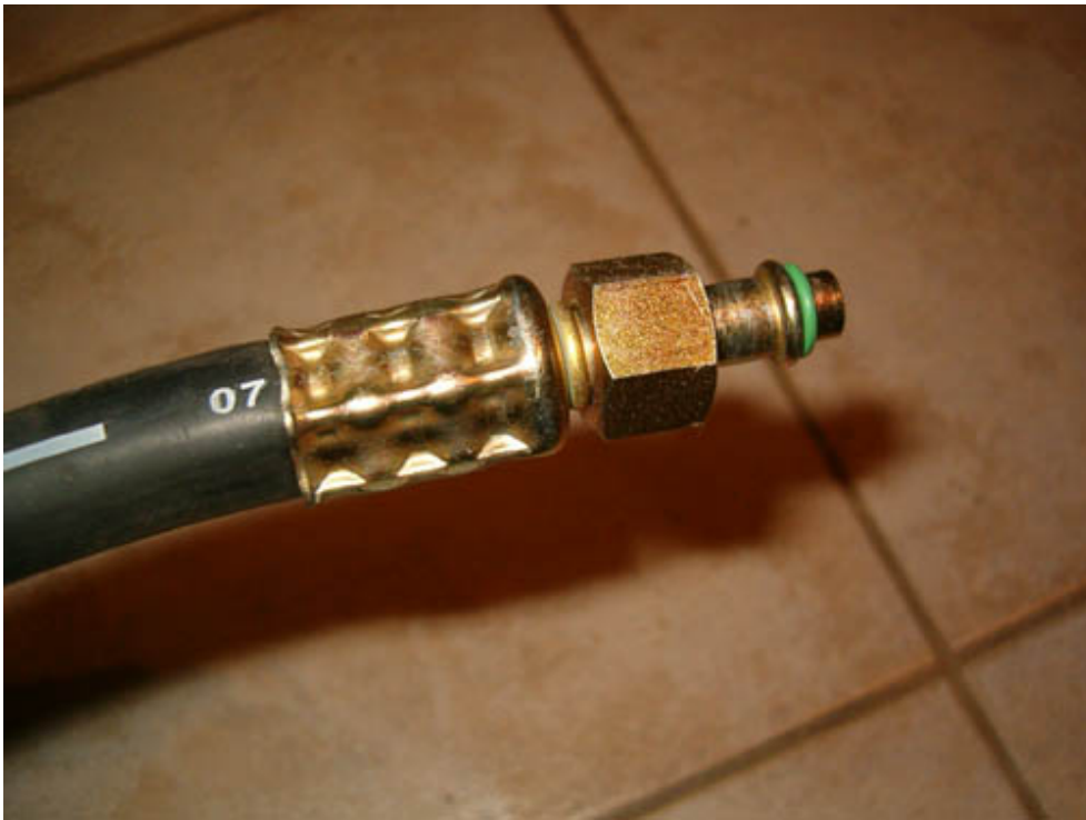
Close up of the new fitting hydraulically crimped to the hose. It surely looks like new.
