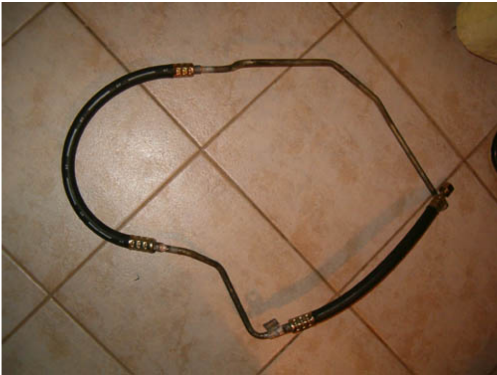
New hose connecting right condenser to drier filter.
