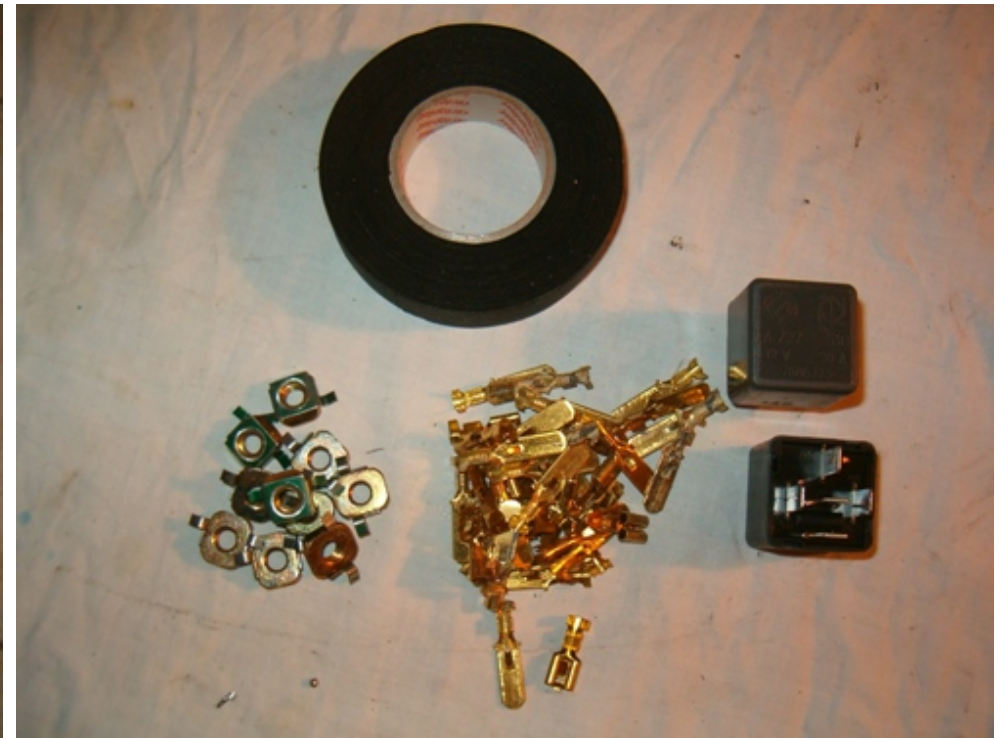
Cloth tape along with new spade connectors and relays. The harness taken from the donor car did not have any relays, so I got two new ones from Alfa. Notice the nuts on the left; these are special nuts from Alfa, required to keep in place pipes etc.
