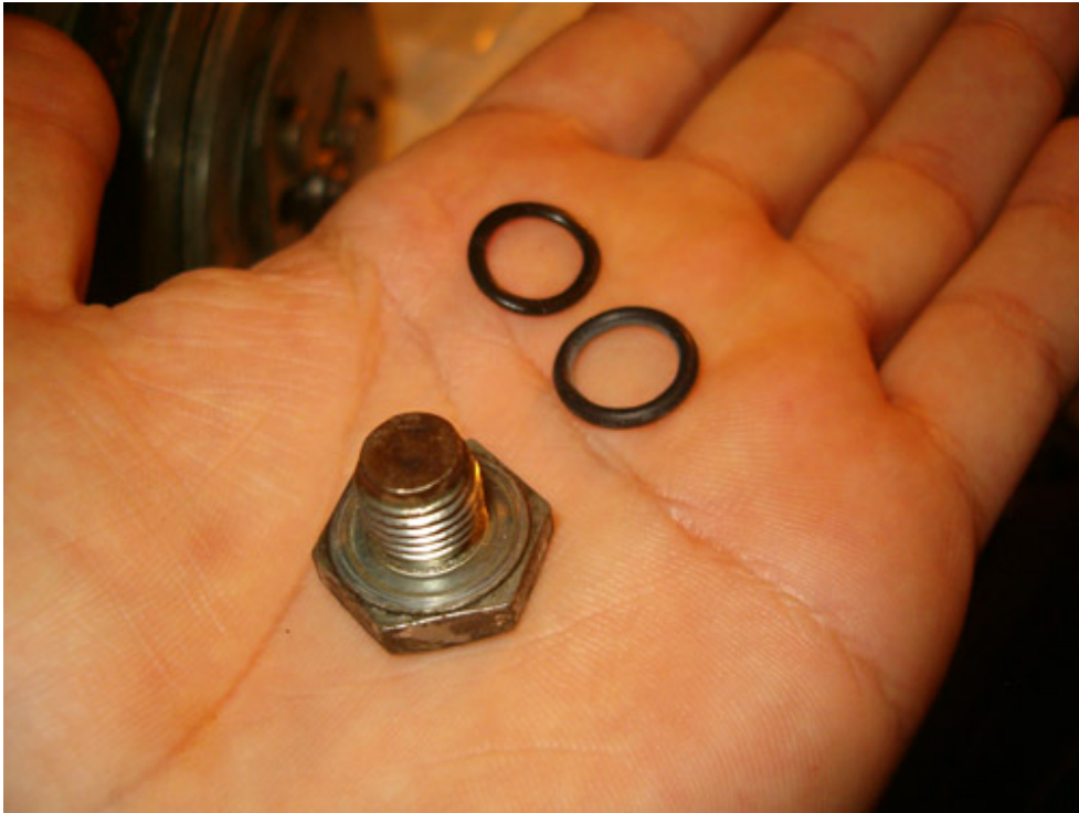
Once you have added oil recover oil drain plug. Be sure to use new O-ring found at the gasket repair kit
