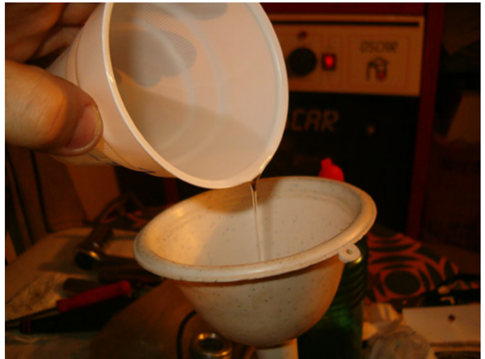
... and using a suitable funnel, pour it slowly to compressor body
