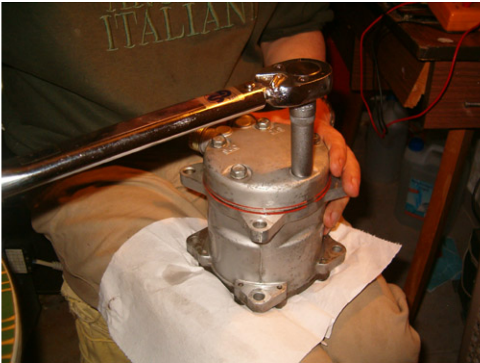
and torque the bolts at 34.3 \pm 4.9 Nm
