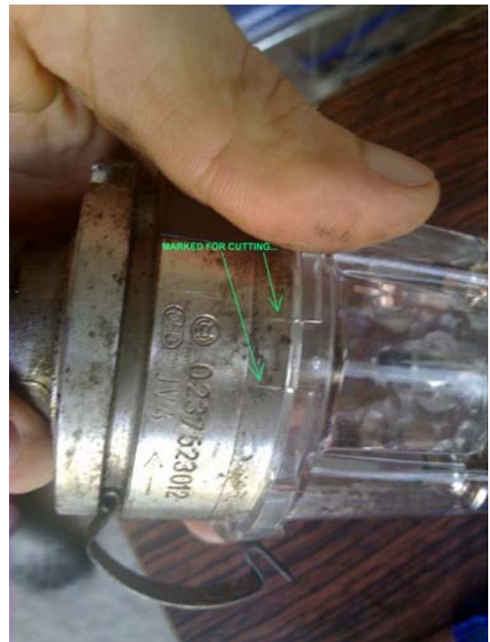
marking the section of the distributor body that need to be machined
