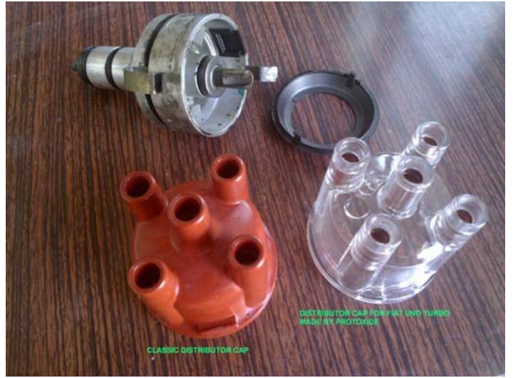
Protoxide cap on the left and original Bosch distributor cap on the right
