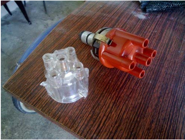
Protoxide cap on the left and original Bosch distributor cap on the right
