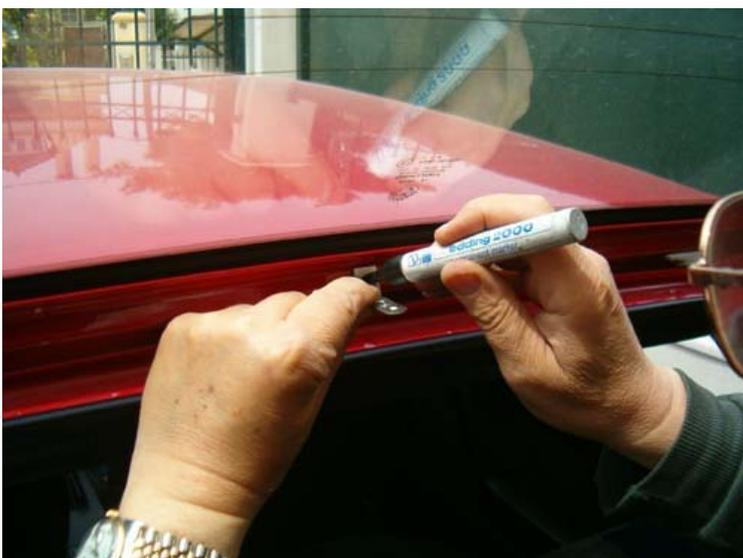
Having measured the centre of the frame, a mark will help drilling
