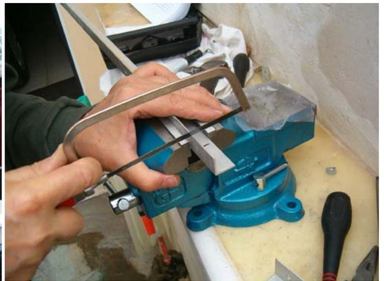
an aluminum piece will help us fabricate two small brackets for the red light. Aluminum is a very nice and handy material to work with; easy cut & easy bent.
