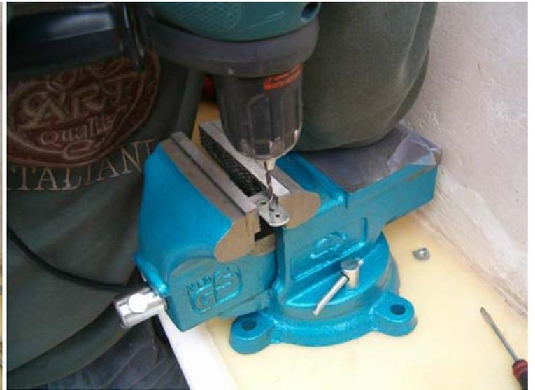
... drilling an extra hole will help us align the bracket to the plate much easier and precisely.
