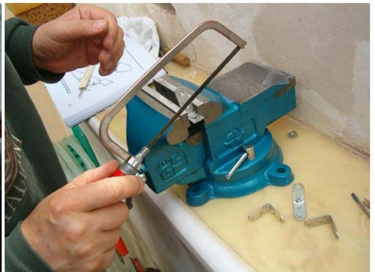
A vice is a must for such cutting jobs - here the bracket is cut to the measured distance
