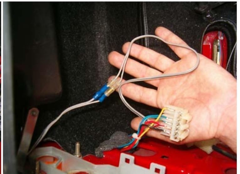
the lead has now reached the rear light and time to wire it up to the electrical system; the white connector you see is for the rear lights. Red and Black leads are intended for the brake light, so I will hook up the supplementary light lead to the above leads.
