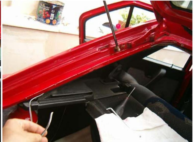
it is now time to pass the lead inside the rubber snorkel and hide it above the headliner
