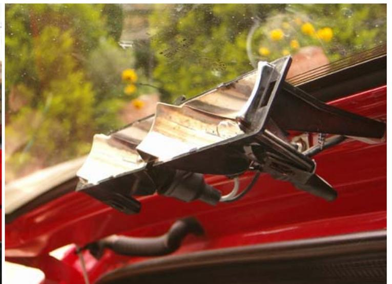
Here you see the light attached to window frame and ready to finalize installation
