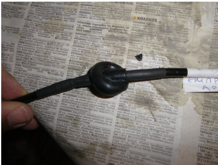
The special rubber grommet off the FORD sensor is used to the Alfa 33 sensor.
